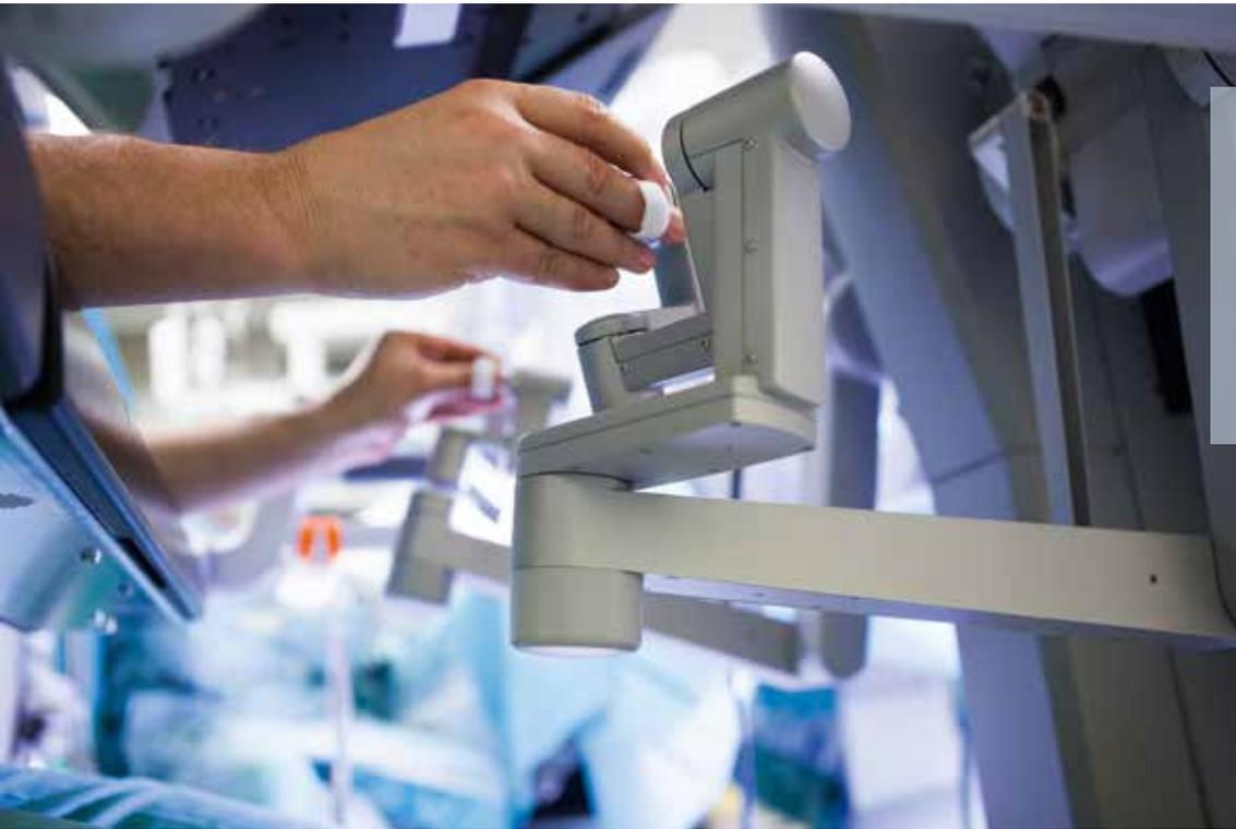
With the Da Vinci operation system, the operator can control the arms and instruments of the robot with millimetre precision using his hands.
