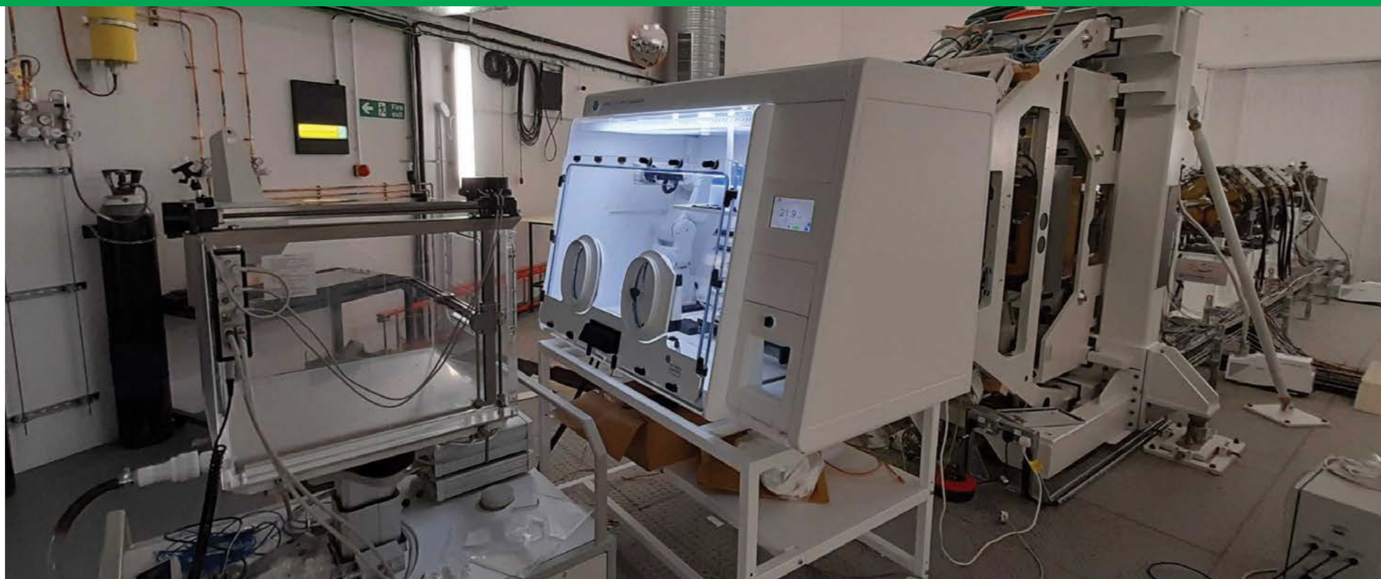
Figure 3 Manchester beam line with hypoxia end station.
